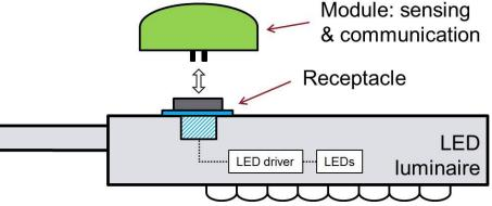
receptacle on the exterior of the LED luminaire and a sensing and communication module (**Precizion**<sup>HALO</sup>) that fits into the receptacle. The standardised interface means that the module can be easily replaced in the field, allowing the luminaire to be upgraded according to new smart capabilities. Also, the luminaire can be shipped with a blank cap in the receptacle, allowing a module to be field-installed at a later date if required.
